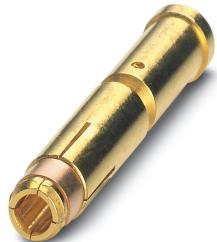
Crimp contact, turned, contact diameter: 2 mm, crimp range: 1.5 mm<sup>2</sup> ... 2.5 mm<sup>2</sup>
